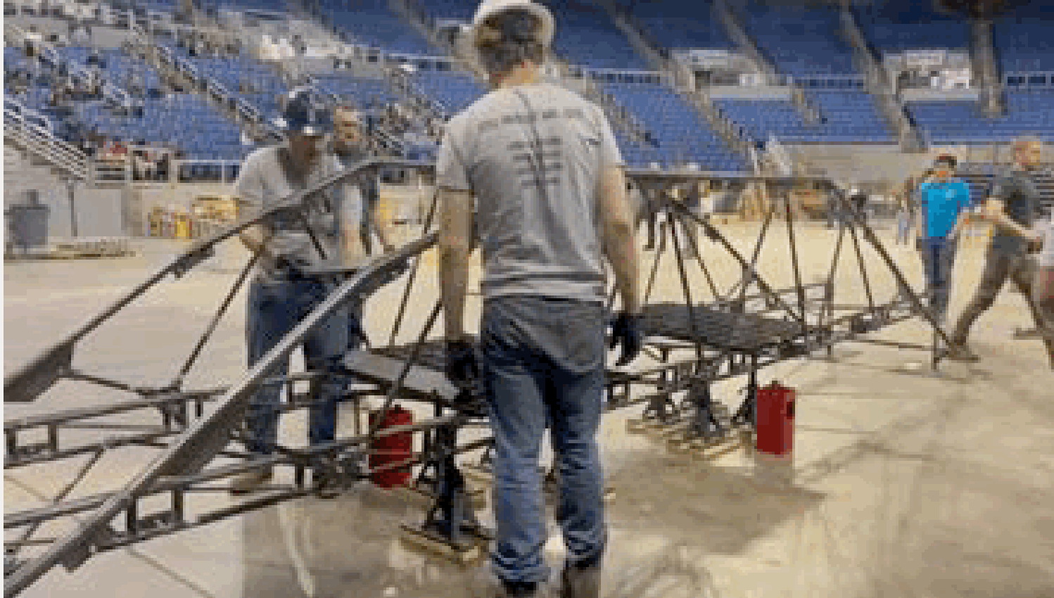
Figure 36.0: Applying Load to Bridge
